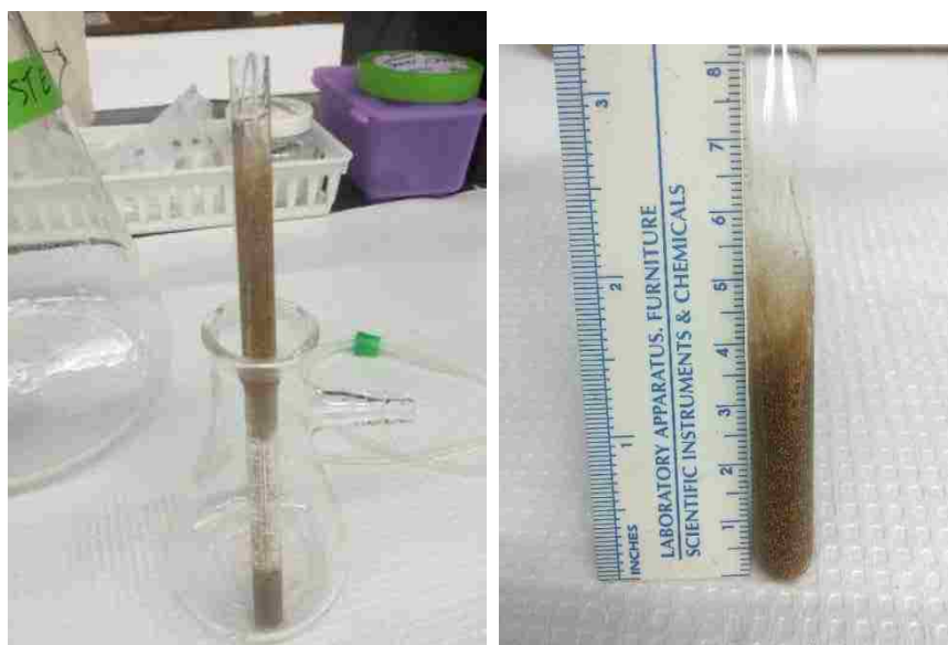
Figure 5.2 Multi-step gravity packing of Artemia embryos after packing into a 10 mm NMR tube with glass wool “cap”
