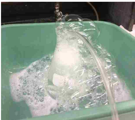
Figure 5.5 Aeration of Tx-100 solution resulting in excessive “foaming”
