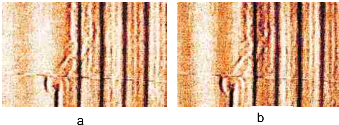
Figure 5.8. Dark-field projections of a 3:1 ABS/ABSFR sample at two consecutive SDD positions. The sample was heated at 275°C. (a) SDD 17.1 mm for correlation length of 1.14 \mu\text{m} and (b) SDD 18.1 mm for a correlation length of 1.21 \mu\text{m} . The residual fringes introduce errors in the measured signal.
