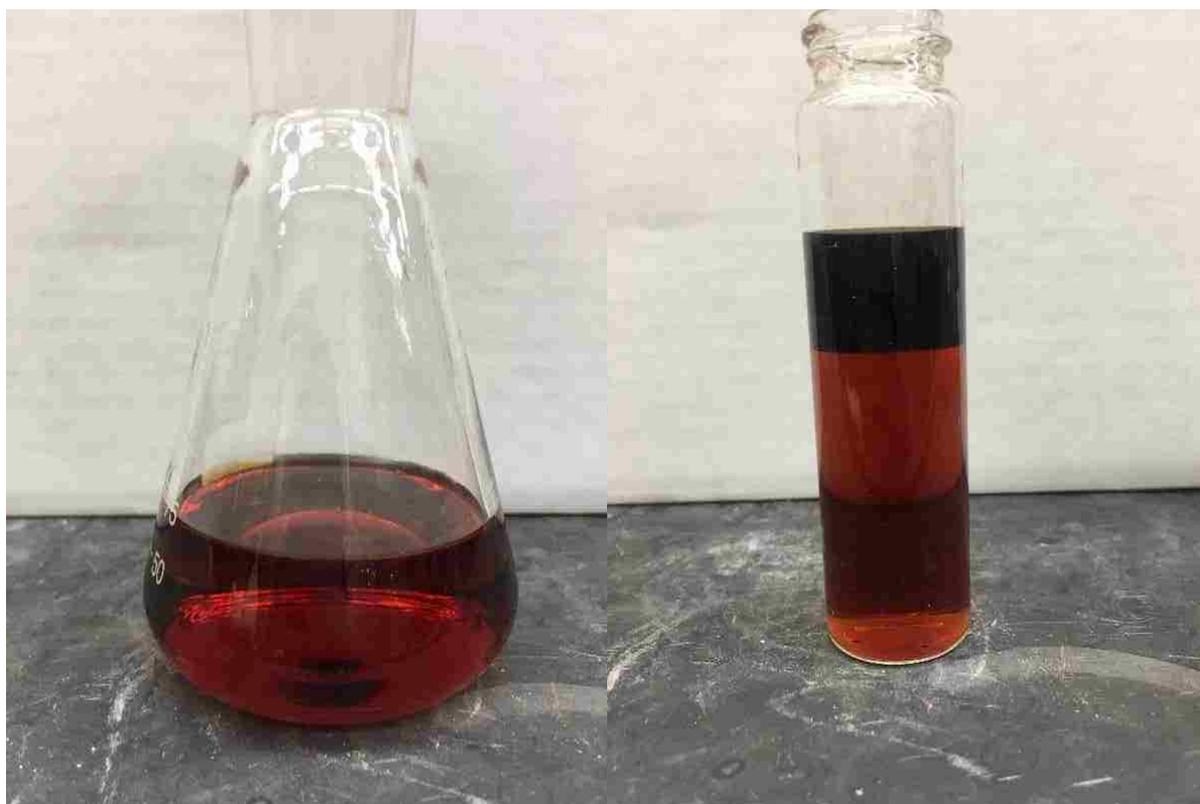
**Figure 3.8.** Catalyst degradation after soaking for 2 hours at  $90^\circ\text{C}$  and 90 psig before reaction (left) and after reaction (right) Aldehyde layer is on top with higher concentration of catalyst, and water/acetone layer on bottom.
