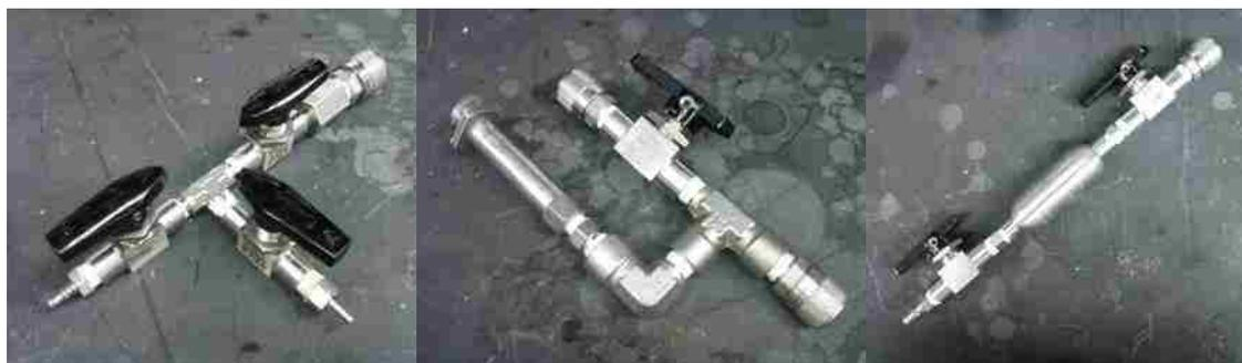
**Figure 3.3.** Autoclave Reactor Arms: Sampling Arm (left), Purge Arm with Pressure Transducer (middle), and Olefin Pressure Injection Arm (right)
