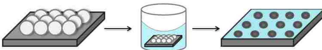
Figure D2 Steps for making nanopores within a thin film of OTS prepared by particle lithography combined with solution immersion. 243 A drop of an aqueous suspension of silica mesospheres in water ( 10 \mu\text{L} ) was deposited on a clean Si(111) substrate. The sample was dried in air for 2 h to produce surface masks. As water evaporated during the drying step, capillary forces pull the mesospheres together to form crystalline layers on flat surfaces. The substrate was placed in an oven at 140 C overnight to temporarily anneal the mesospheres to the surface. After cooling, the sample was immersed in a 0.1% solution (v/v) of OTS in toluene for 5 h to form an OTS film surrounding the surface mask. To remove the mesoparticles, the substrate was sonicated for 15 min in ethanol and water successively. The sample was dried under argon before characterization with FMM-AFM.
