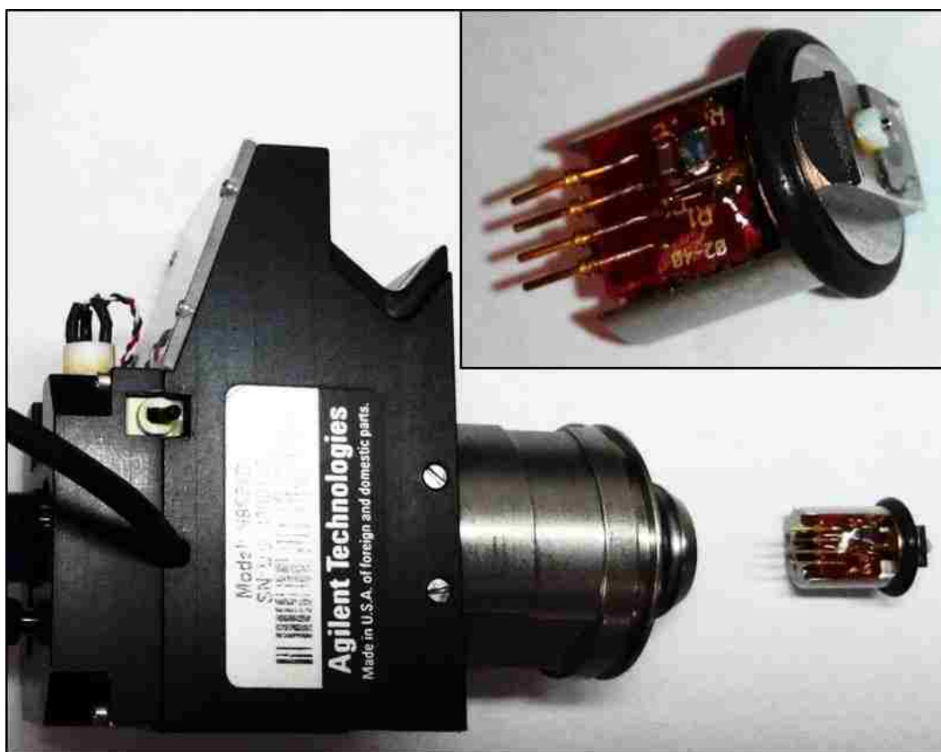
Figure B1 Scanner and nose assembly for STM. Insert is the STM nose assembly.
