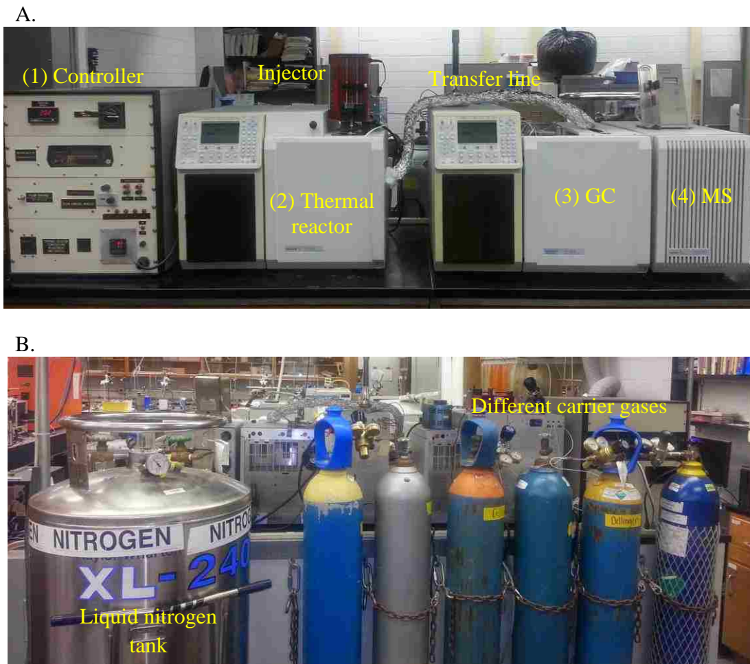
Figure 2.1 System for thermal diagnostic studies (STDS) A. Front and B. Back.
