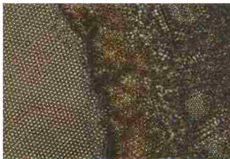
Figure 2.6: Close packed mesospheres on glass. Oil immersion micrograph (100×).
