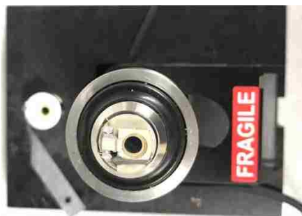
Figure 2.8 Piezo tube scanner with DLFM nosecone attached
