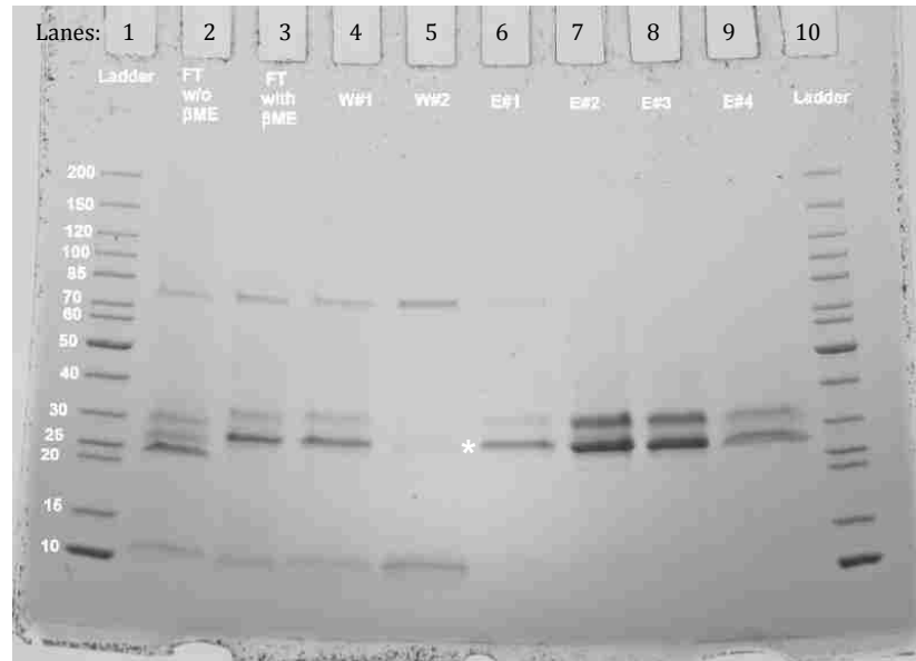
Figure 17. SDS-PAGE gel image of the nickel affinity chromatography gravity purification of pLIC-EGF27-TEV-EGFP-His after TEV cleavage using AcTEV protease. Lane 1 and 10 (protein ladder), lane 2-3 (flow-through with and without \beta ME), lane 4-5 (washes), and lane 6-9 (elutions).
