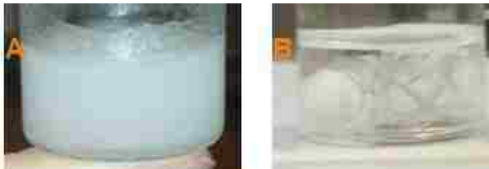
Figure 2.2. Crystallization of a DES by A) stirring and B) after sitting with a stir bar present.
