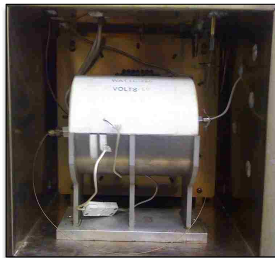
Figure 2.3 Inside view of the reactor and furnace housed within a GC oven
