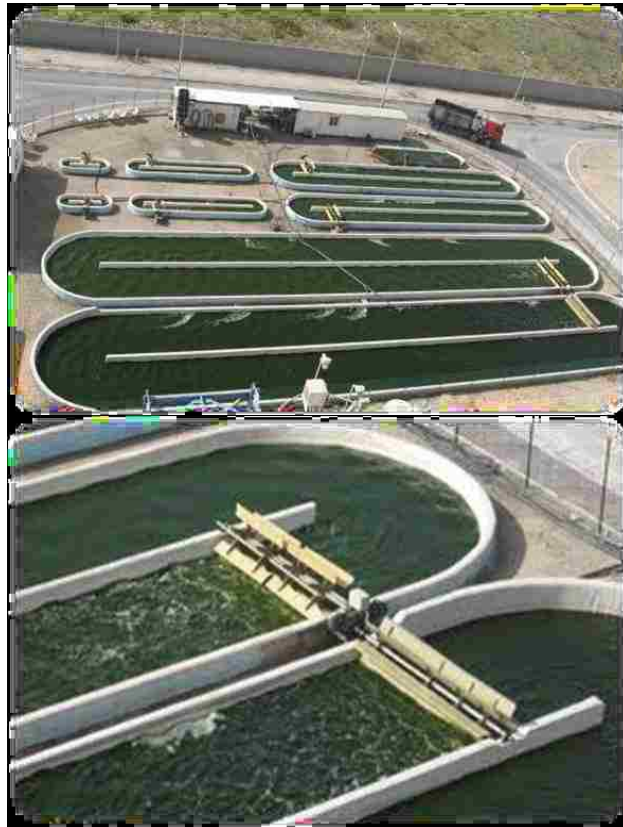
Fig. 1.3 Open ponds/raceways used for microalgal cultivation 63
