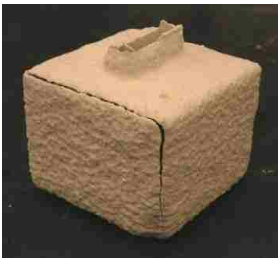
Fig. 10. Example of crack formed in the shell during pattern removal.
