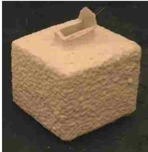
Figure 1. Shell built around foam pattern: 50.8 x 63.5 x 63.5 mm.
