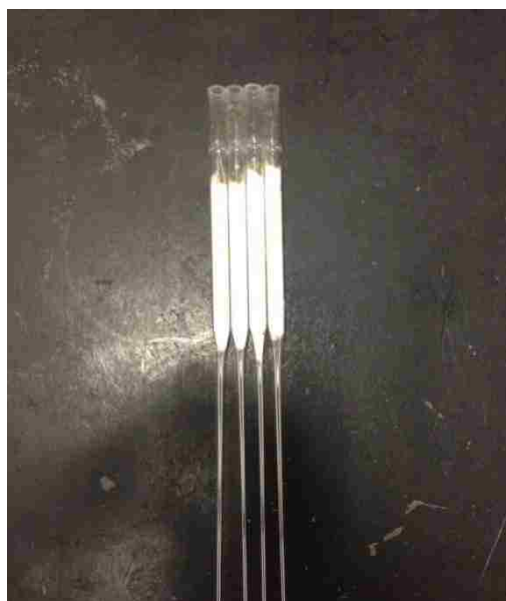
Figure 1 Scheme of the lab prepared SPE silica gel columns
