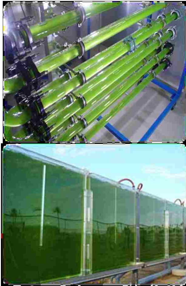
Fig. 1.4 Closed photobioreactors used for microalgal cultivation 58
