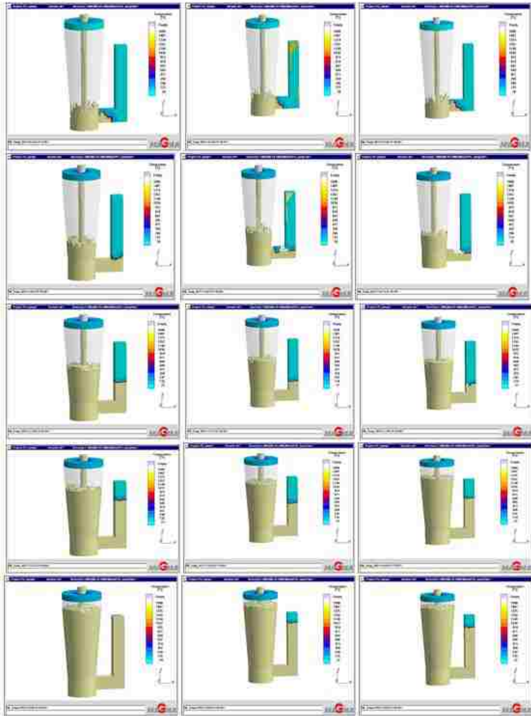
Figure 2 The resulting temperature distribution of the melt and receding polystyrene foam at a particular time (0.5, 1.7, 2.8, 3.9, and 5s, respectively from top to bottom). The density of polystyrene was 25, 57, and 73Kg/m 3 , respectively from left to right. The coating thickness was 0.1mm.
