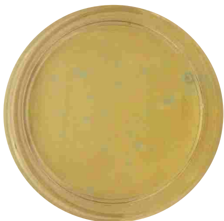
Figure 1-5. Petri dish with urea-urease clock reaction and universal indicator. Red/orange color (pH <5.5), yellow (~pH 6.5), blue green (pH >8). Blue green fronts spontaneously occur and propagate throughout the dish.
