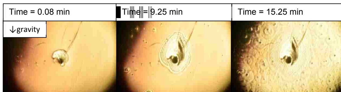
Figure 3-26: Schlieren Images of Exp. 7. This experiment contained 0.05 M ETTMP, 0.075 M PEGDA, 0.03 M urea, 0.93 mg/mL urease, 9% (v/v) universal indicator, and initiation of fronts in center with already reacted urea-urease solution (pH 9). Also, the petri dish was tilted 10°.
