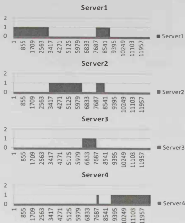
Figure 5-17: Partial Storage of Four Cloud Servers After Running SPRT.
