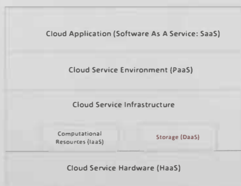
Figure 1-1: Cloud Computing Services Architecture.
