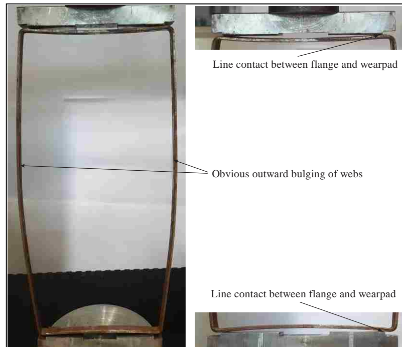
Figure 55: Obvious deformation of webs and flanges of RHS ring between wearpads
