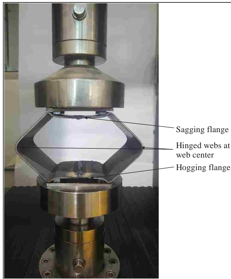
Figure 72: Hinged webs and bent flanges of RHS piece between wearpads
