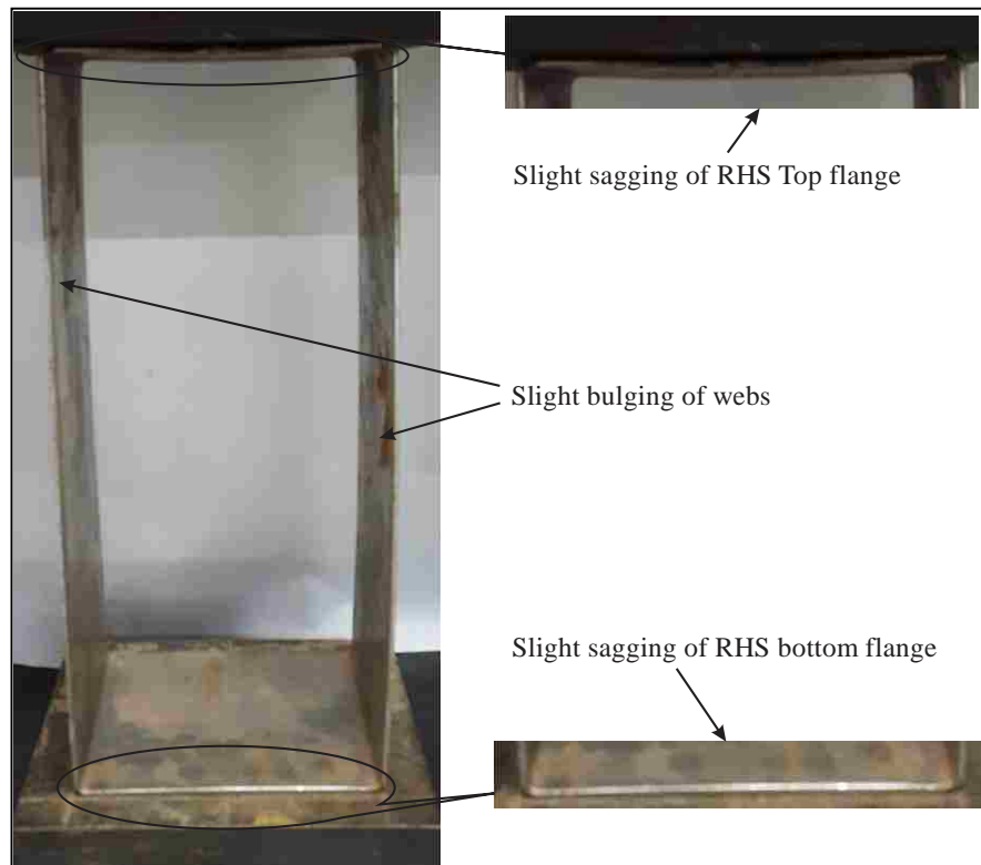
Figure 62: Initiation of bending of flanges and bulging of webs of RHS piece between platens
