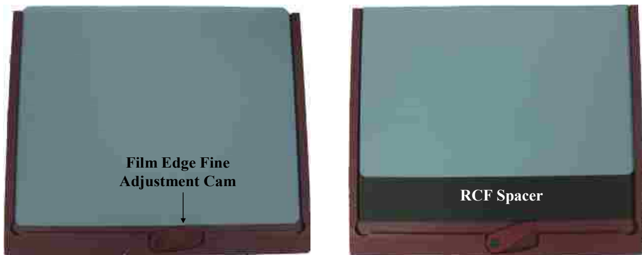
Figure 2.4: Third prototype film cassette. The film edge can be displaced \leq 3.7 cm to allow precise alignment of the film edge with the phantom surface for different sized films. A spacer was used for RCF to account for the films' shorter length.
