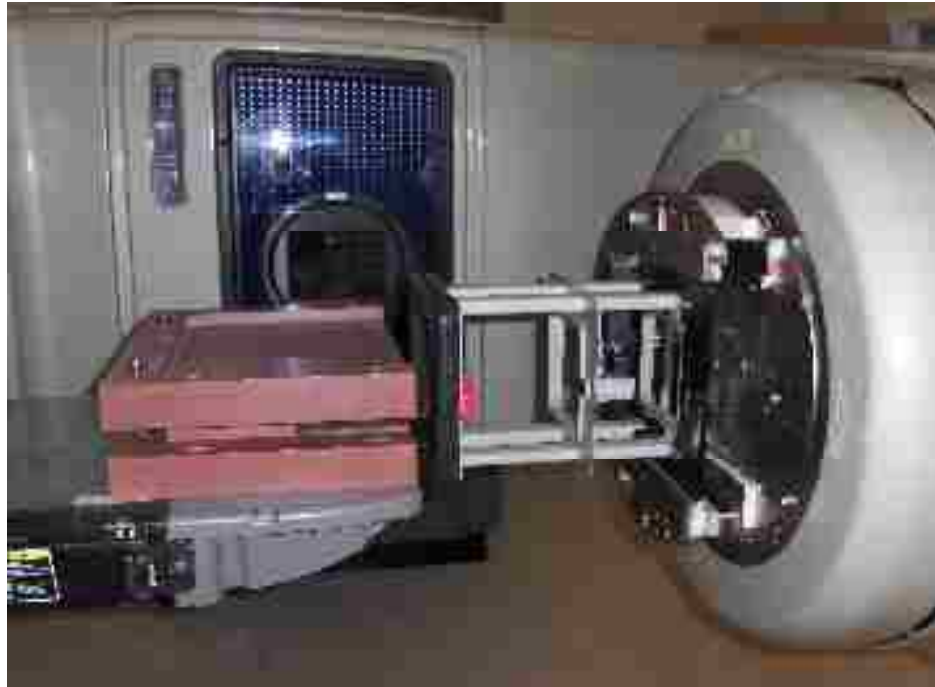
Figure 2.3: Second prototype film phantom measurement set-up. The cassette was placed between the two slabs of phantom housing. The gantry was rotated to 90^\circ and the couch was placed at 270^\circ .
