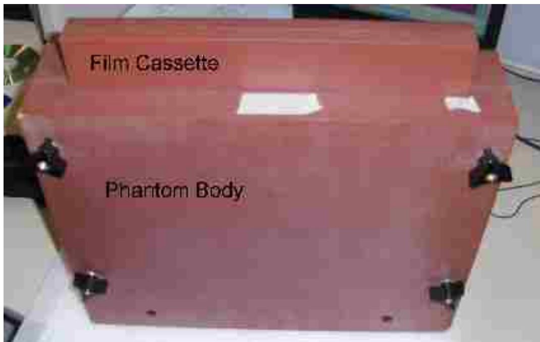
Figure 2.1: Picture of the first prototype showing the film cassette and phantom body.
