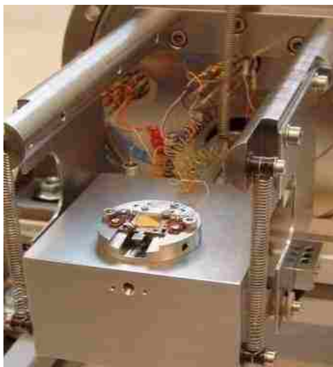
Figure 2.14 Aarhus STM. STM is on the Aluminum block which is suspended by the three springs.
