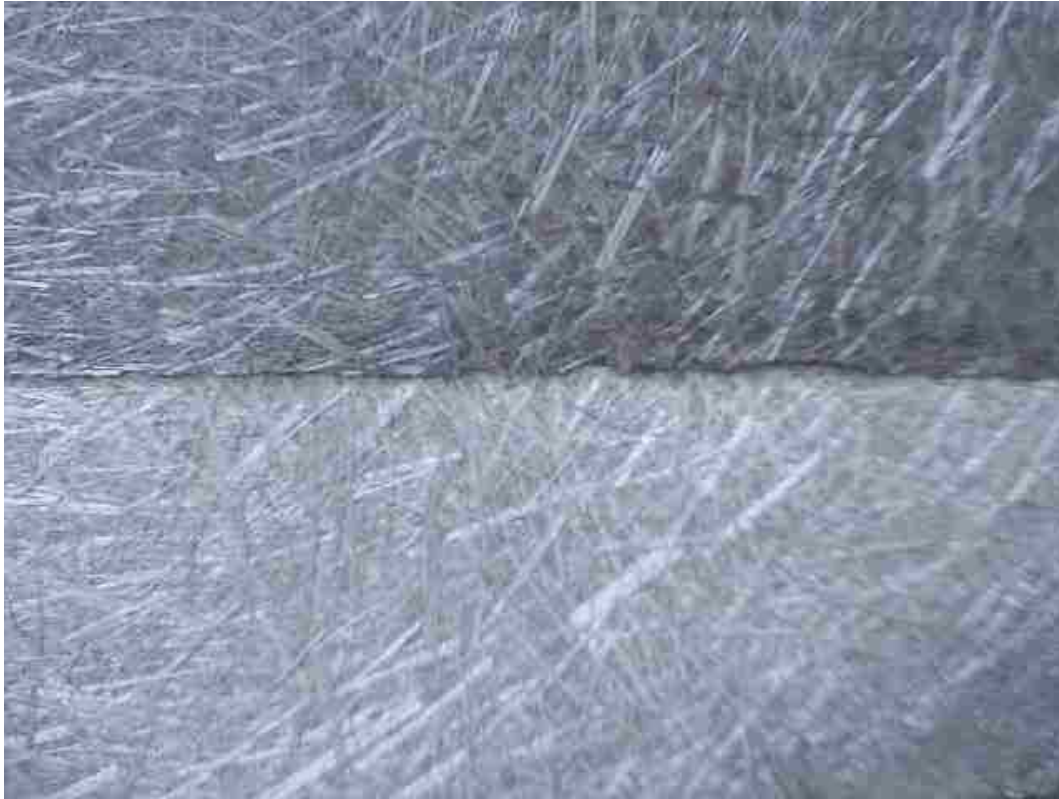
Fig: 2.7 Mo- coated C fibers produced by JW Composites LC.
