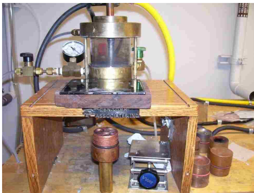
Fig: 2.3 Arc melting chamber and copper hearth.
