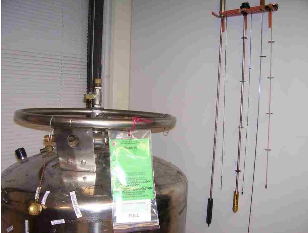
Fig: 2.12 Liquid He tank and other tools for sample installment inside the PPMS.
