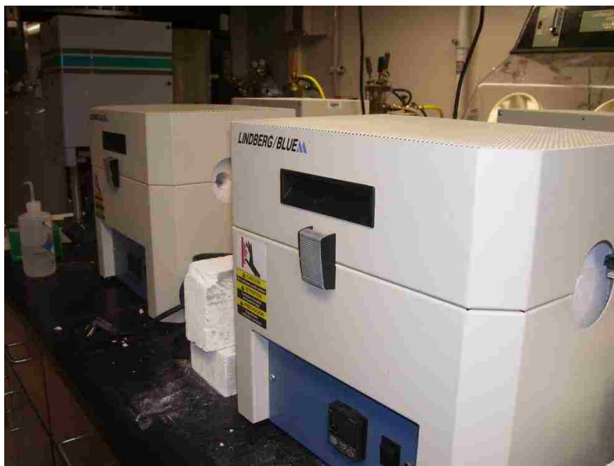
Fig: 2.2 High temperature tube furnaces used to anneal the samples.
