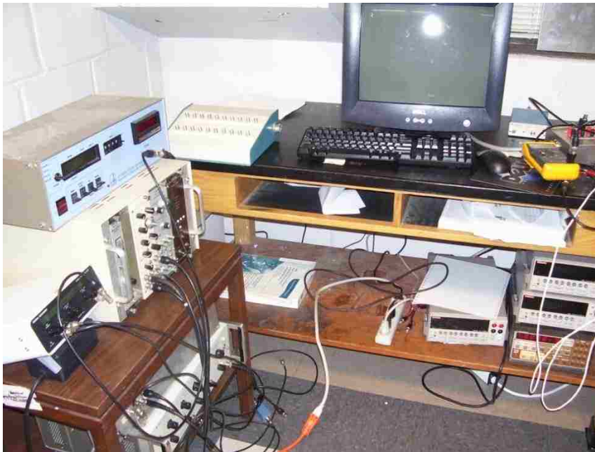
Fig: 2.14 Equipments for the measurement of critical current density.
