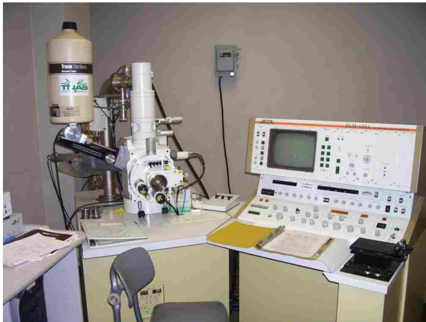
Fig: 2.10 JEOL 840A Scanning electron microscope in the geology department at LSU.
