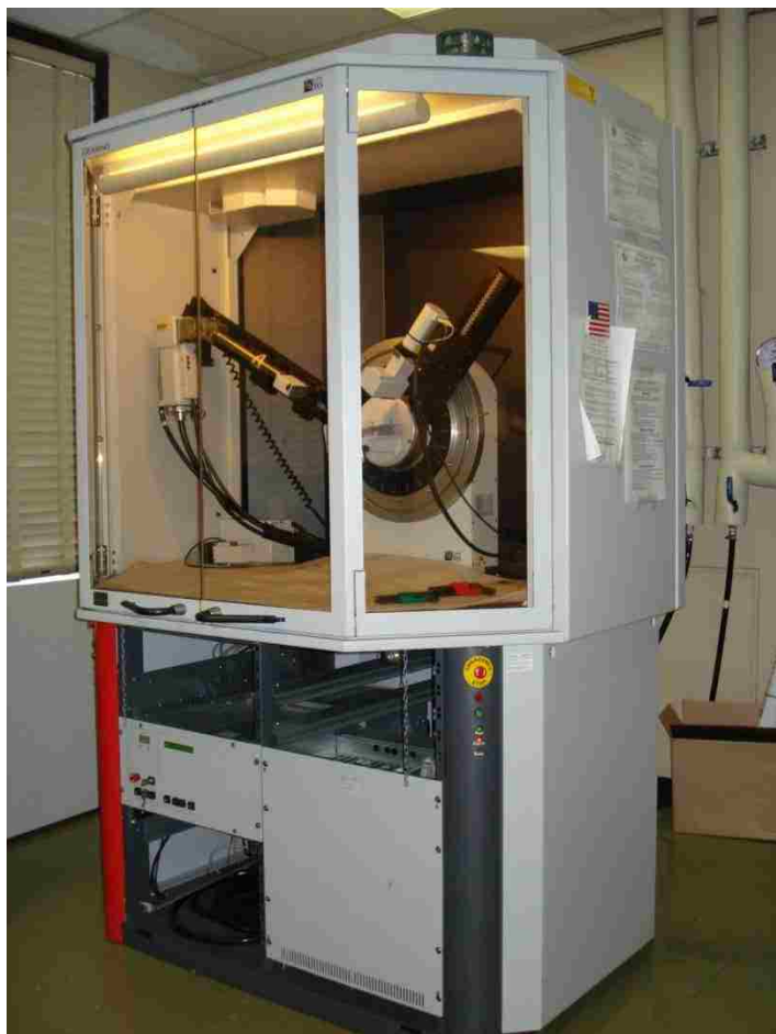
Fig: 2.8 A Bruker D8 Advance Powder Diffractometer housed at Chemistry department.
