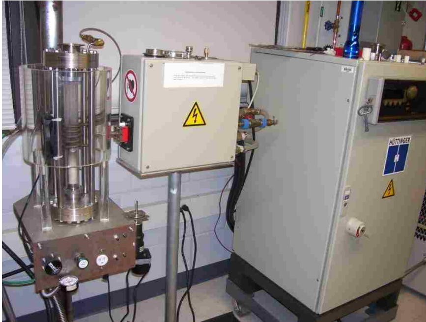
Fig: 2.4 RF induction melting system.
