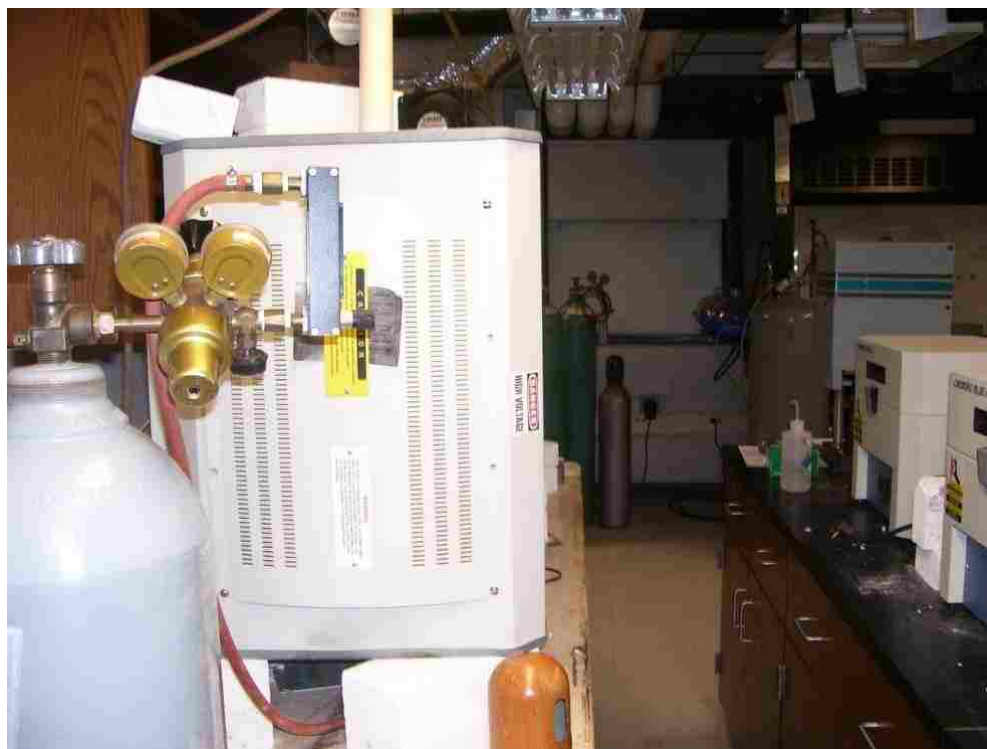
Fig: 2.5 High temperature vertical furnaces used for single crystal growth.
