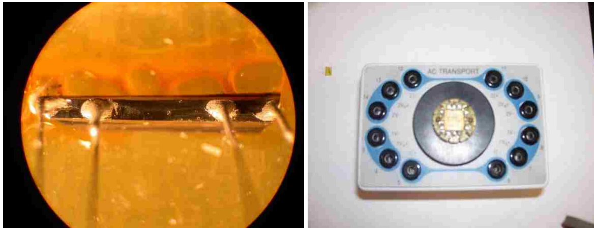
Fig: 2.13 Single crystal with four current and voltage leads and Samples puck and base for Ac transport.
