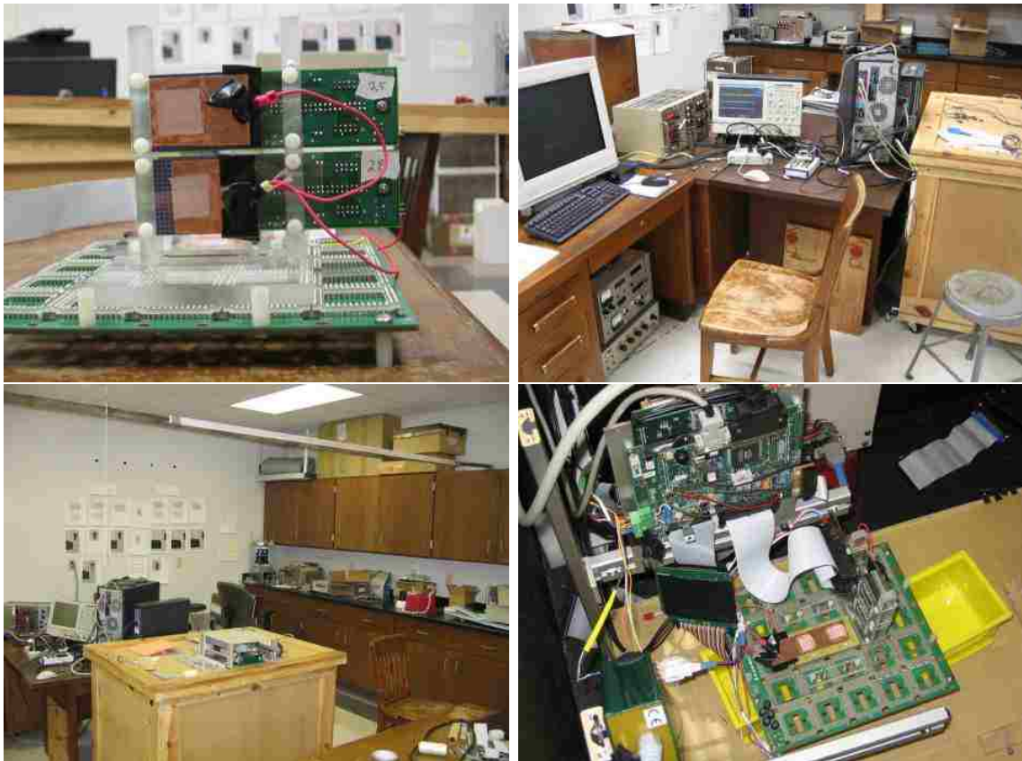
Figure 4.1. The L shaped prototype detector. The photos show the mounted detector modules (top left), workstation (top right), external reference frame and light tight box (bottom left) and the assembly inside the light tight box.
