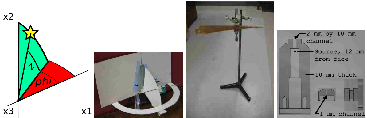
Figure 4.4. From left to right, local co-ordinate system, pointing device, source stand and cylindrical collimator with end pieces.
