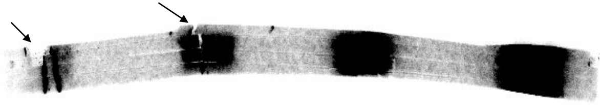
Figure 47. Image of storage phosphor strip flattened and held against artery plaque phantoms for a 2 minute acquisition time. The size of each plaque phantom was 4 x 6 mm, the volume of FDG deposited was 4 \text{ mm}^3 and the activities from left to right were 4.0 nCi, 12.8 nCi, 38.6 nCi, 126.4 nCi. Arrows indicate damage to the phosphor layer, likely due to handling while putting the flattened tips on the readout drum.
