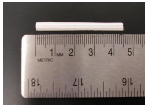
Figure 15. Flattened storage phosphor detector tip with four segments.
