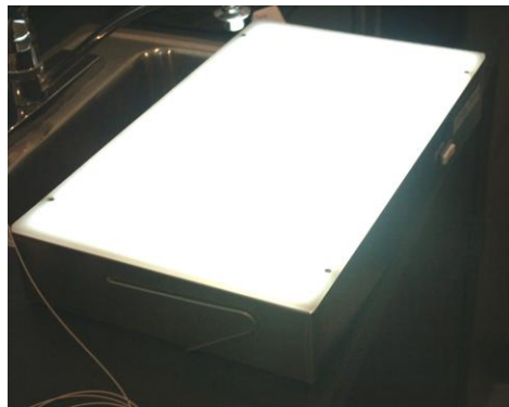
Figure 22. The Porta trace 1118 flat panel white light source produces a 30 W flood of light, used for erasing storage phosphor plates.
