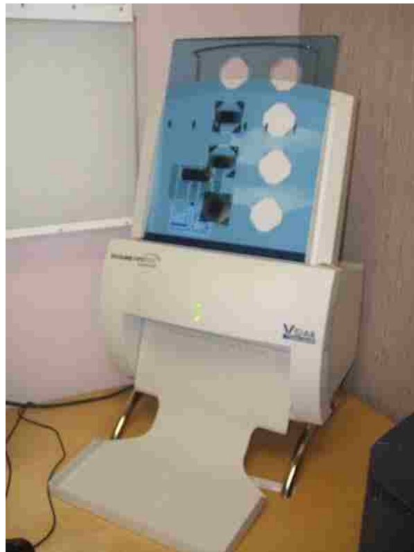
Figure 17. Vidar Dosimetry Pro 16-bit film scanner; Film digitization template is shown prior to scanning.
