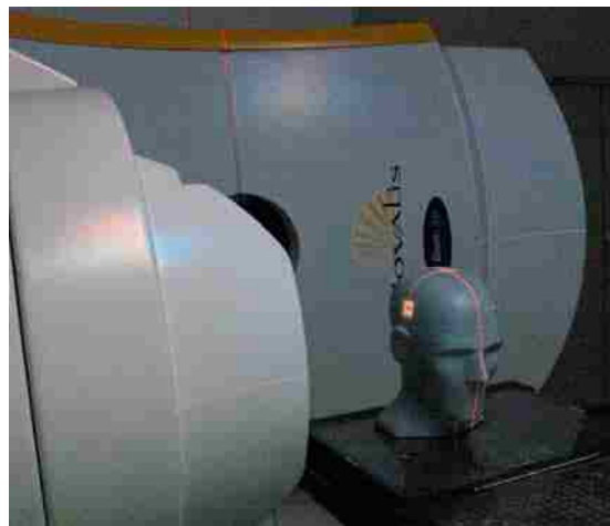
Figure 32. View of gantry and phantom for precision test for sagittal film.
