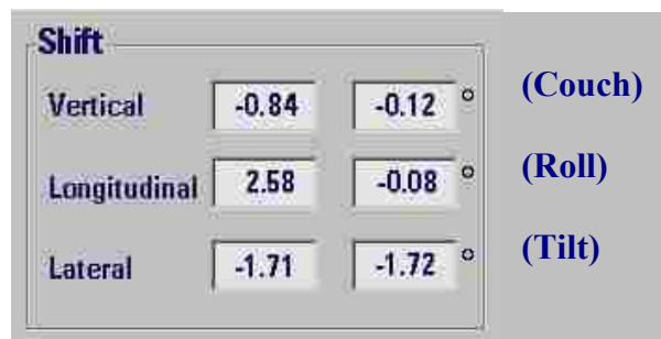
Figure 39. ExacTrac Shift Report. Each of 6 dimensions can be corrected by the shifts shown.
