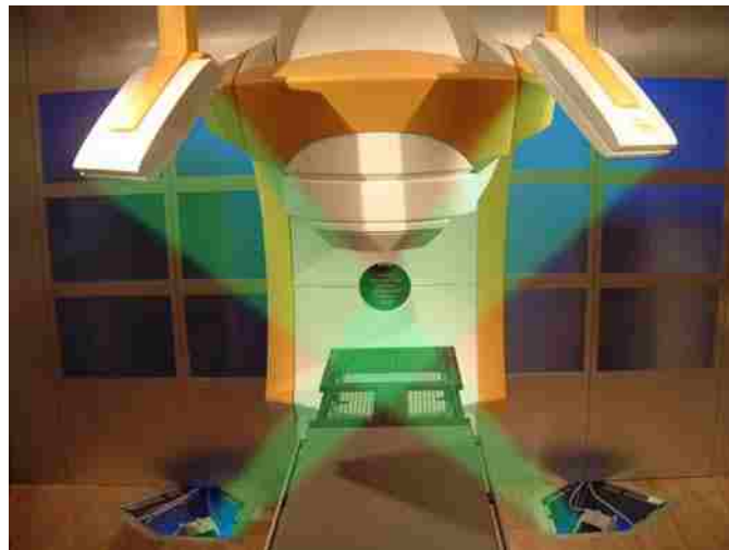
Figure 4. ExacTrac X-ray beams. X-rays are directed through isocenter to the flat panel detectors. X-ray tubes shown here with covers removed.
