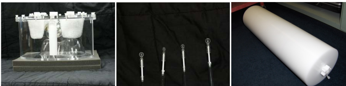
Figure 4: Pictured from left to right: The anthropomorphic torso phantom, a sample of micro hollow spheres used to simulate lesions, and the scatter phantom.
