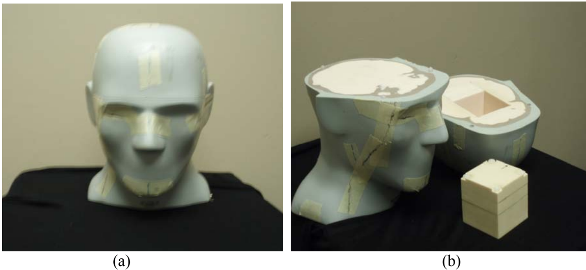
Figure 2.1: (a) CIRS Model 605 Head Phantom. (b) Film phantom measurement system with film block.
