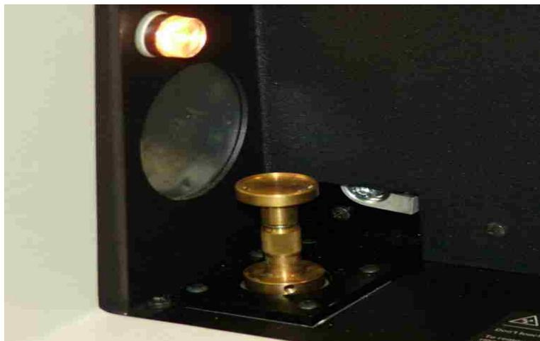
**Figure 16: Skyscan-1074 imaging compartment. Samples are placed on the stage (pedestal in image center) which rotates. The x-ray tube (not shown) produces a “cone” of x-rays which travel from right to left. The scintillator is located behind the circular mylar-covered window at left.**
