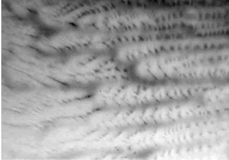
**Figure 18: Skyscan-1074 open field. The pixel values representing photon counts are displayed in grayscale. Tube settings were 40 kVp, 1000  $\mu$ A, 420 ms exposure time, 100% gain. This open field image is an average of five acquisitions.**
