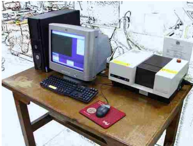
**Figure 15: Skyscan-1074 Portable X-ray Microtomograph system (right) connected with a desktop computer for image acquisition.**
