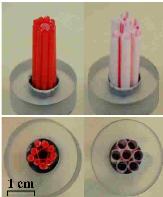
Figure 31: Top and side views of the polypropylene (left) and HDPE (right) tubes arranged in the PMMA base for imaging.
