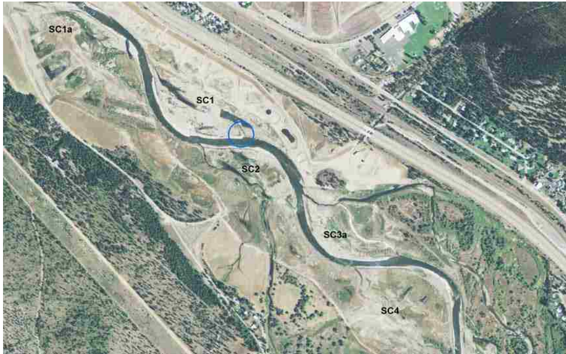
Figure 4.9. Restoration area with locations of key secondary channels indicated. The blue circle indicates a potential avulsion node, which is based on a comparison of bed slope gradients of the primary and secondary channels.
