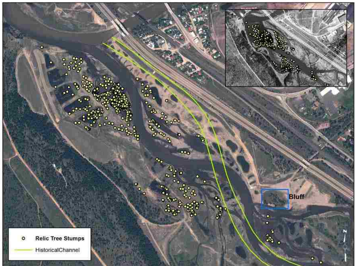
Figure 4.5. Distribution of tree stumps and proposed historical channel alignment. The large map plots relic tree stumps against the current channel as well as a hypothesized historical channel. For reference, the inset map depicts tree stumps against the river before dam removal. The proposed historical configuration is based on the distribution of tree stumps and sedimentological data collected from 2003 to 2005. Sediment cores obtained from the area between the eastbound and westbound lanes of Interstate 90 (immediately adjacent to the floodplain) did not contain any alluvium, suggesting it is unlikely the historical channel occupied that portion of the valley. The blue box indicates the presence of a bluff \approx 15-20 m high. The historical channel – consistent with GLO and USGS maps – was likely straighter than today’s river, but still exhibited hallmarks of a meandering planform (cf. Woessner, 1995).
