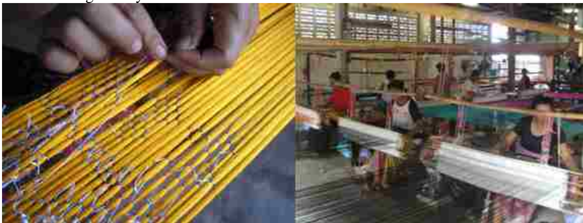
Figure 1.3: (a) detail of tie-dying threads before they are woven into mudmee fabric; (b) a silk weaving factory in Chonnabot.
