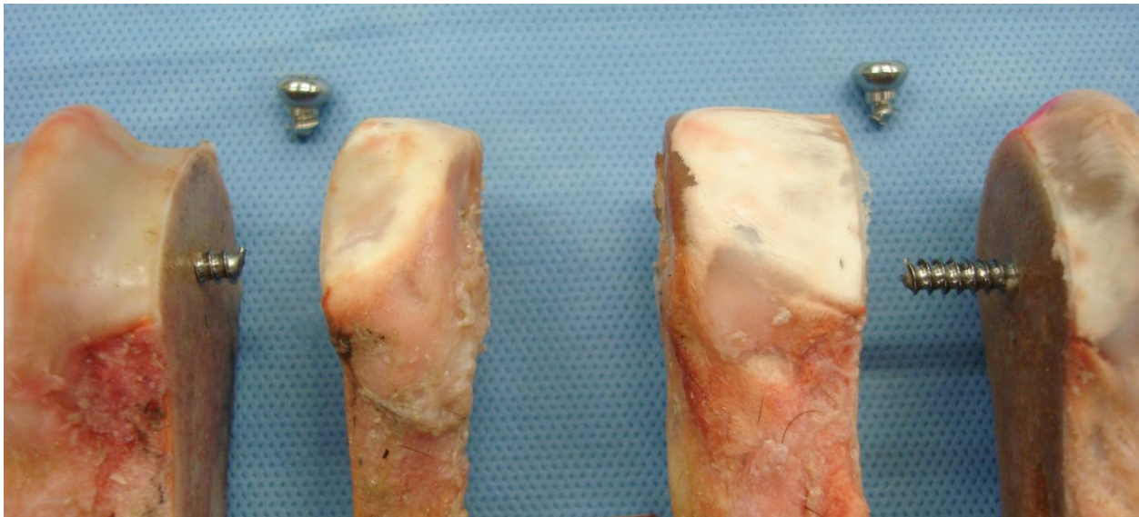
Figure 3.1 Equine cadaveric third metacarpal bones that were tested for torque to failure of experimentally created medial condylar fractures of various thicknesses repaired with a 4.5 mm AO screw placed in lag fashion. Types of failure that can occur with repair of condylar fractures include bone failure with the threads stripping or screw failure with the screw breaking at the screw head junction.
