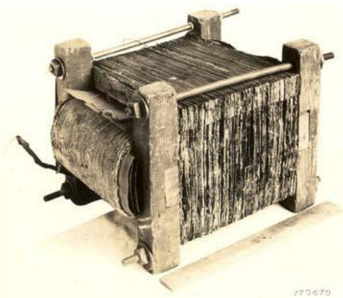
Figure 2.3. Stanley's first transformer which was used in the electrification of Great Barrington, Massachusetts in 1886 [13]
