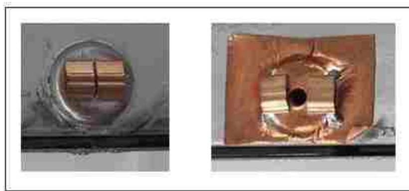
Figure 4.2. Gaskets connections on back panel for better contact to back cover
