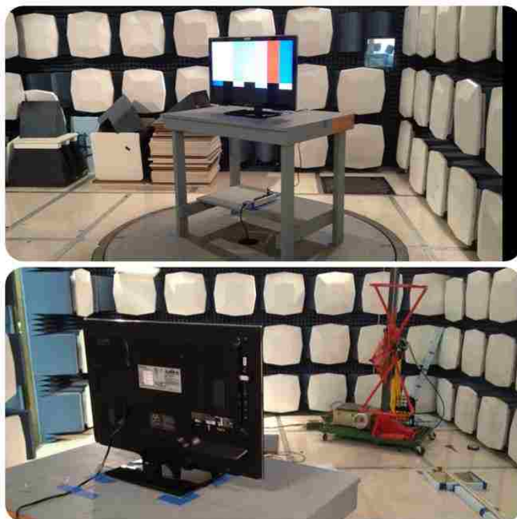
Figure 2.3. Radiated emissions test setup
