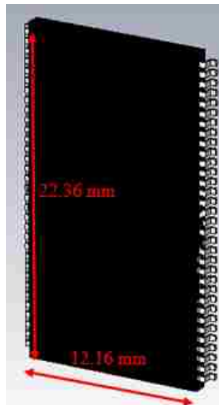
Figure 5.5. Package model of the IC
