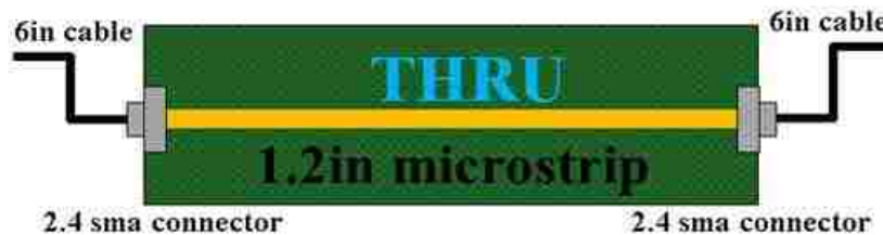
Figure 4.6. Geometry Model of the Microstrip
