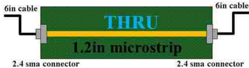
Figure 1.4. Geometry of the DUT Structure
