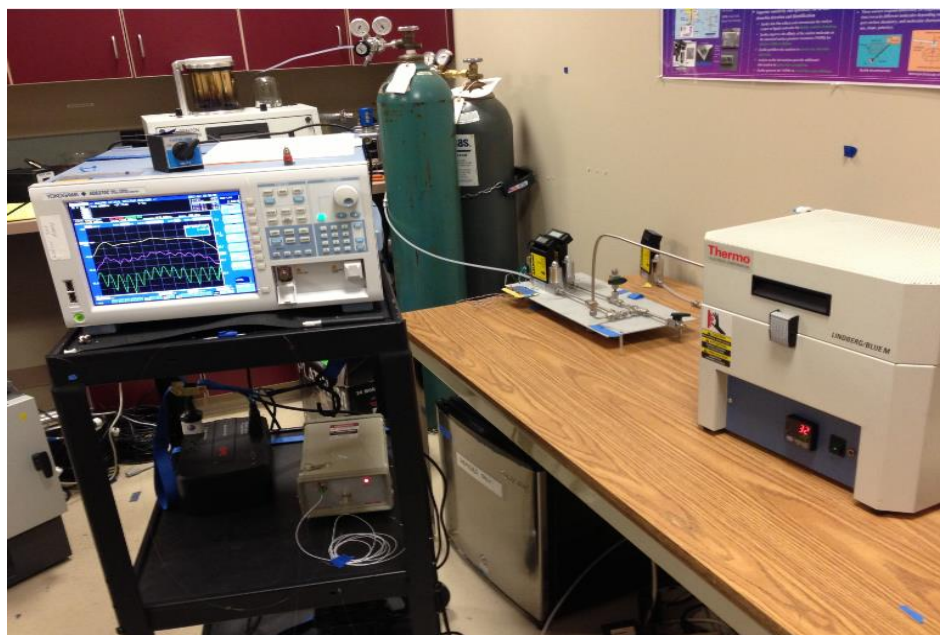
FIGURE 3.4. EXPERIMENTAL SET-UP FOR REGENERATION OF IONIC LIQUID
