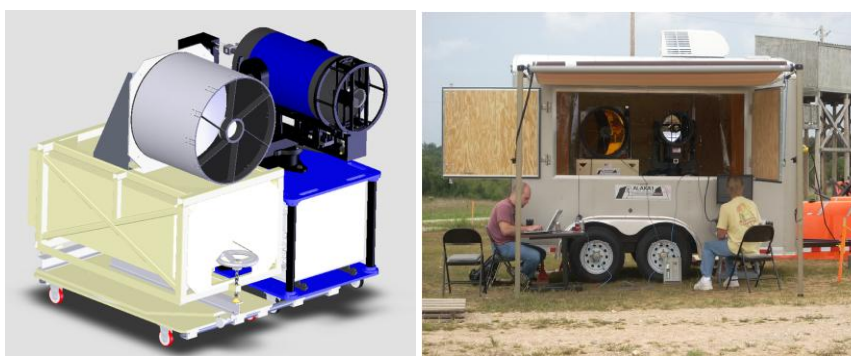
(a) Model of TREDS-2 TEPS/Raman system (b) TREDS-2 in a field test
