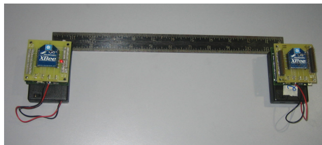
Fig. 10. UMR-SLU G4-SSN motes arranged for creating spatial diversity with a separation of 25 cms
