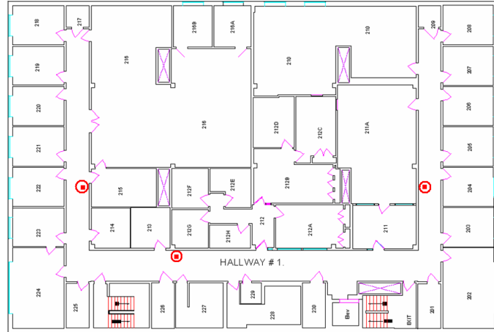
Fig. 12. Floor plan of ERL second floor. Receiver pair positions are marked with circled squares
