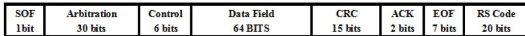
Figure 4.8 Extended CAN Frame with Individual Fields and RS-Bits Shown. Frame used for HARQ Type-I R-S20/CRC
