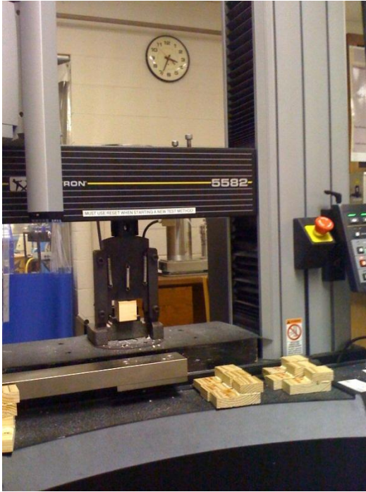
Figure 2 The Instron with the ASTM D143 attachment with a sample loaded.
