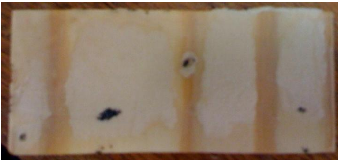
Figure 34 The wood that was used in a thin layer test. The lighter areas were able to support a front while the darker areas were not. The layer of adhesive applied was thin enough to make out the different regions in the wood.
