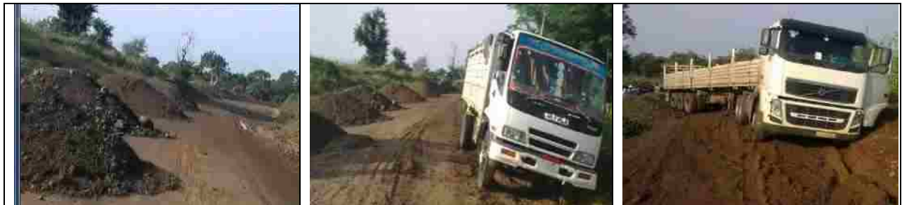
Figure 7. 4: Accidents Caused by Lack of Timely Maintenance and Improper Dumping of Gravel (Corridor 1 Near GelagoTown)
