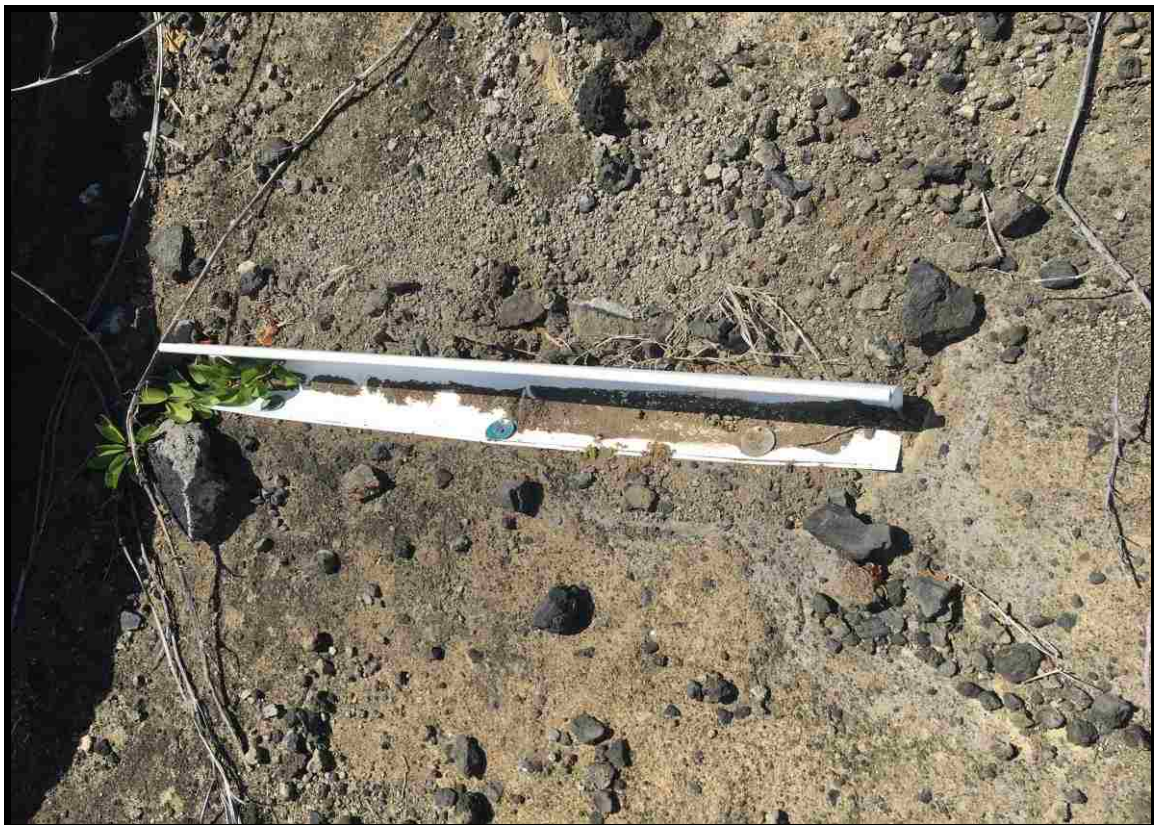
Figure 3.3b: Gerlach trough with captured sediment.
