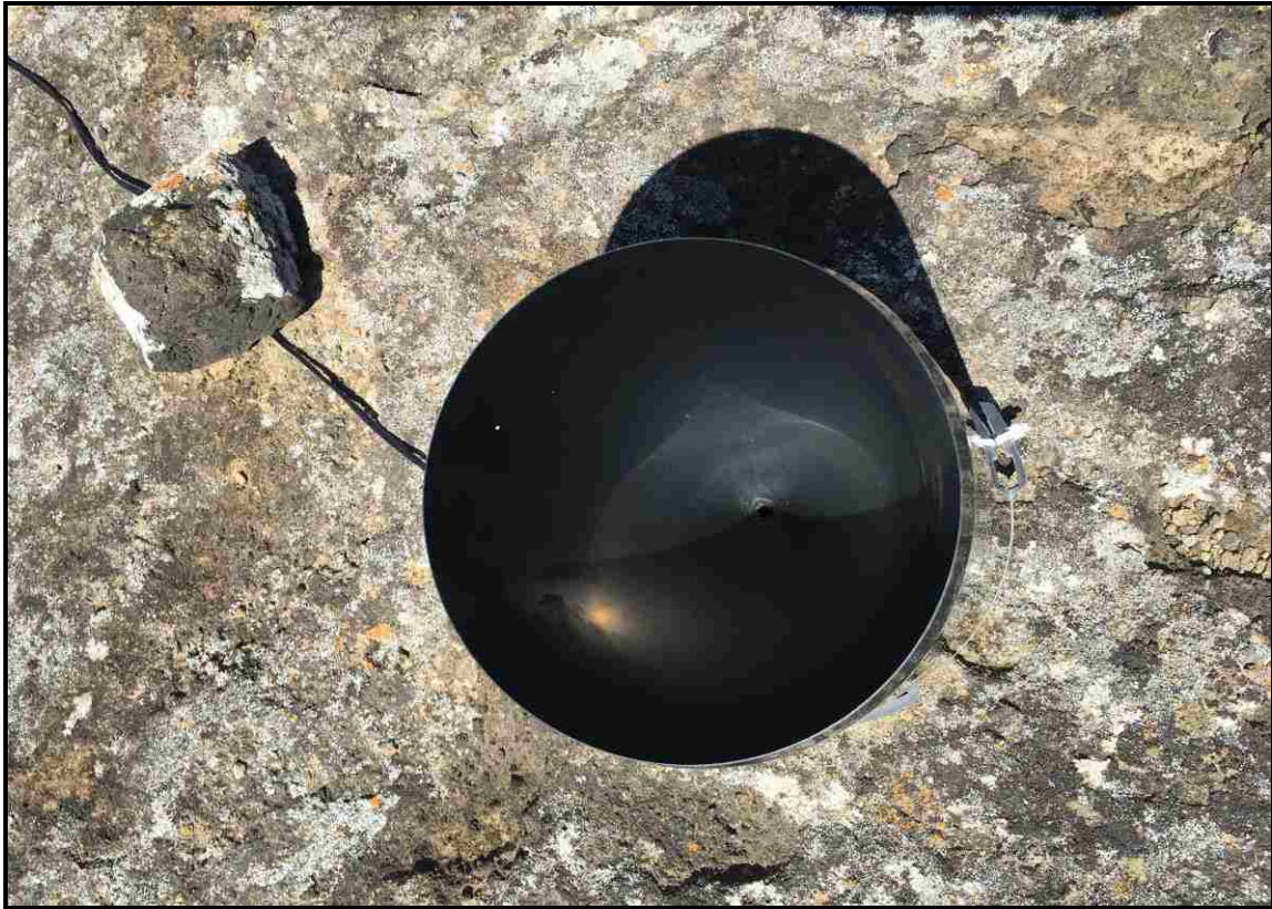
Figure 3.2: Automatic rainfall tipping bucket (0.2 mm resolution) attached to environmental monitoring station.
