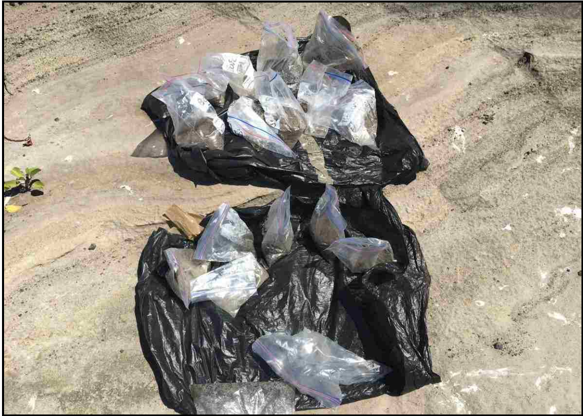
Figure 3.4: Monthly sediment samples stored in bags for analysis. Wet sediment was left to dry in the sun for several hours.
