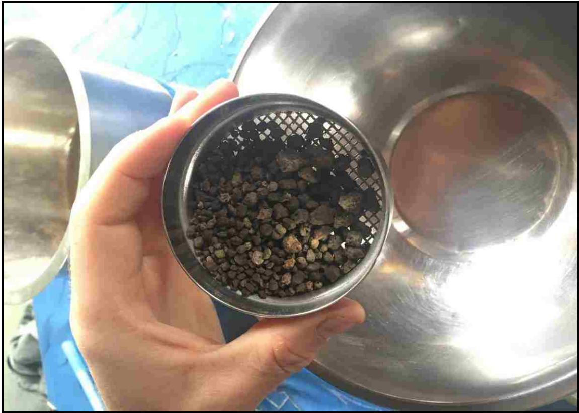
Figure 3.7: Particle size analysis using 2 mm sieve. Note, a large amount of gravel left behind.
