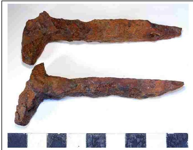
Fig. 6 Hand-forged nails with square shanks # DWA209IR/F10//MO5.
