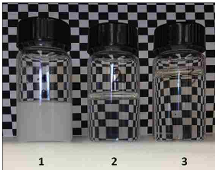
Fig. 3: Vial 1: CUP solution of Poly-1 before filtering; Vial 2: CUP solution of Poly-1 after filtering; Vial 3: CUP solution of Poly-5 (MW = 15K)
