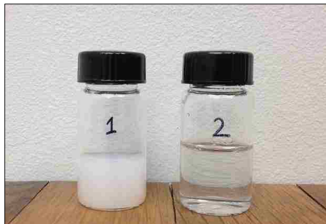
Figure 6. Water reduction in presence of 50 ppm calcium for 1) CO 2 H-copolymer 2) SO 3 H-copolymer
