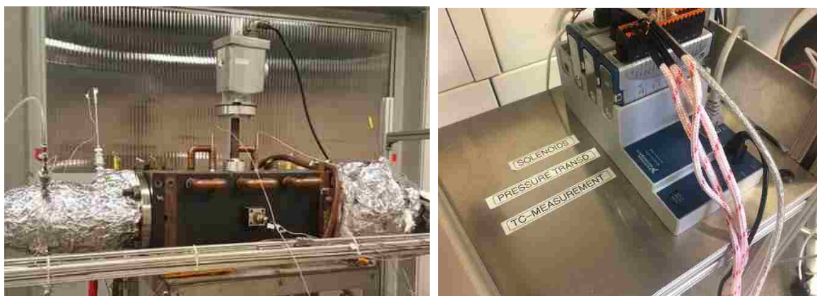
Figure 2.2. The DAQ system (Right) and the Thermocouples Distribution Along the Heater/ Reactor (Left)
