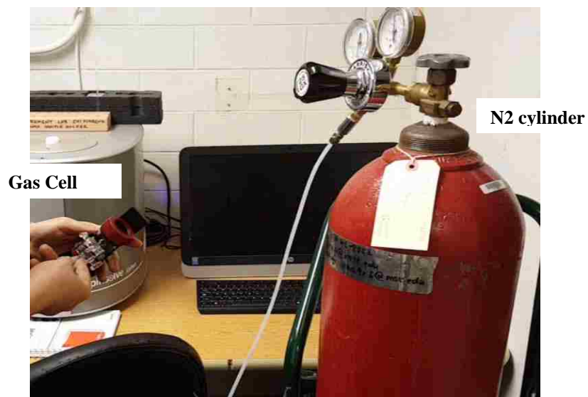
Figure 3.12. Purging the gas cell by using N 2
