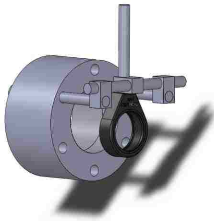
Figure 2.11. The lens mounting system for the laser ablation source.
