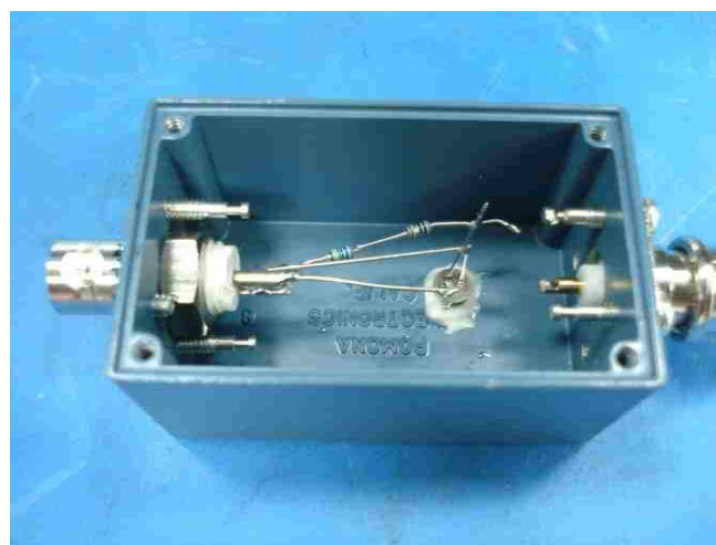
Figure 6-3: Internal photo of National Semiconductor LM34 based temperature sensor. The LM34 can be seen glued to the base of the metal Pomona® box with thermal epoxy.
