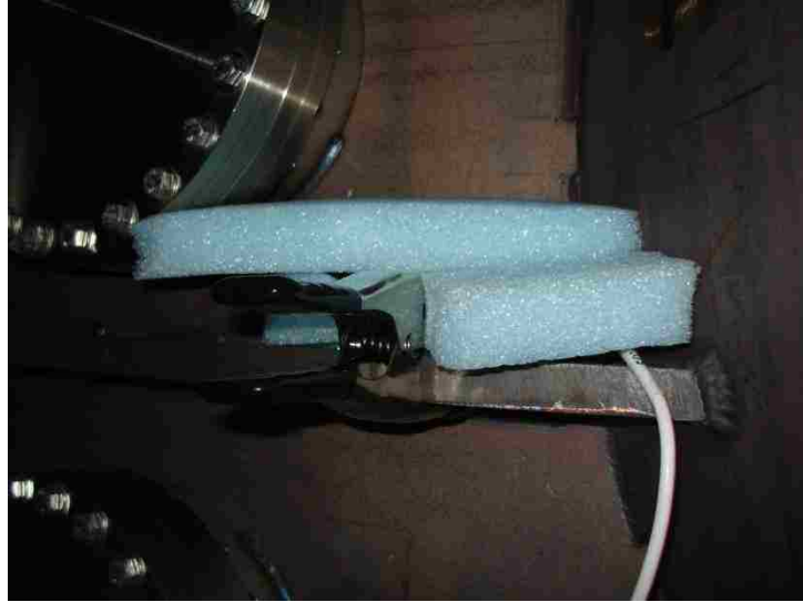
Figure 6-4: Photograph of a thermal sensor situated on a BSC shell.
