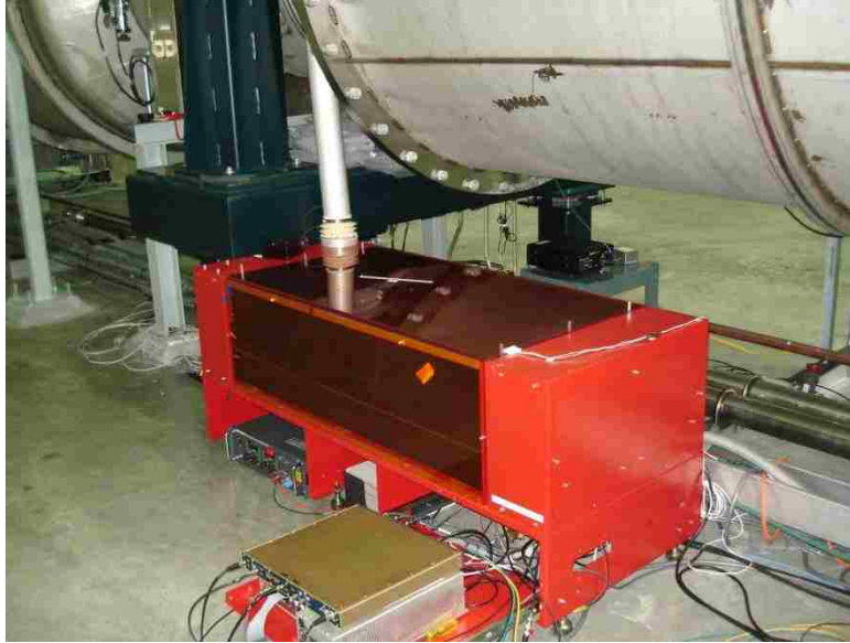
Figure 1-7: An photograph of a TCS laser table taken at Livingston Observatory. The orange box contains a 35 W CO 2 laser that is shaped into a spot or an annulus and projected onto the ITM 15 m away via the vertical launch tube. The steel tube adjacent the TCS bench is the vacuum envelope. The green pedestal at 10 o'clock is an optical lever pier.
