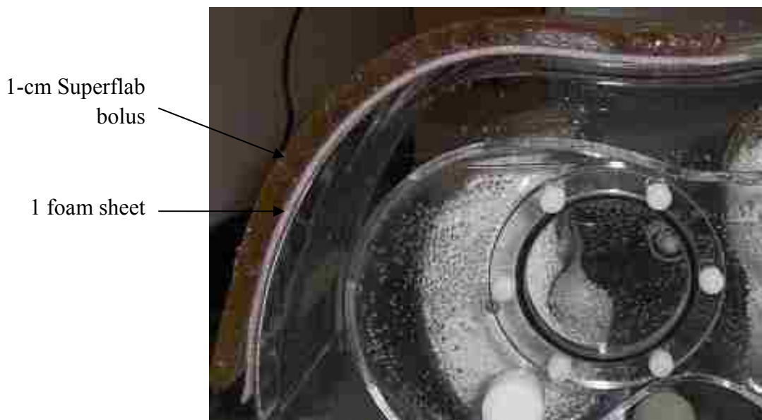
Figure 2.21. Foam cushioning material was placed between Superflab and phantom surface to simulate an air cavity
