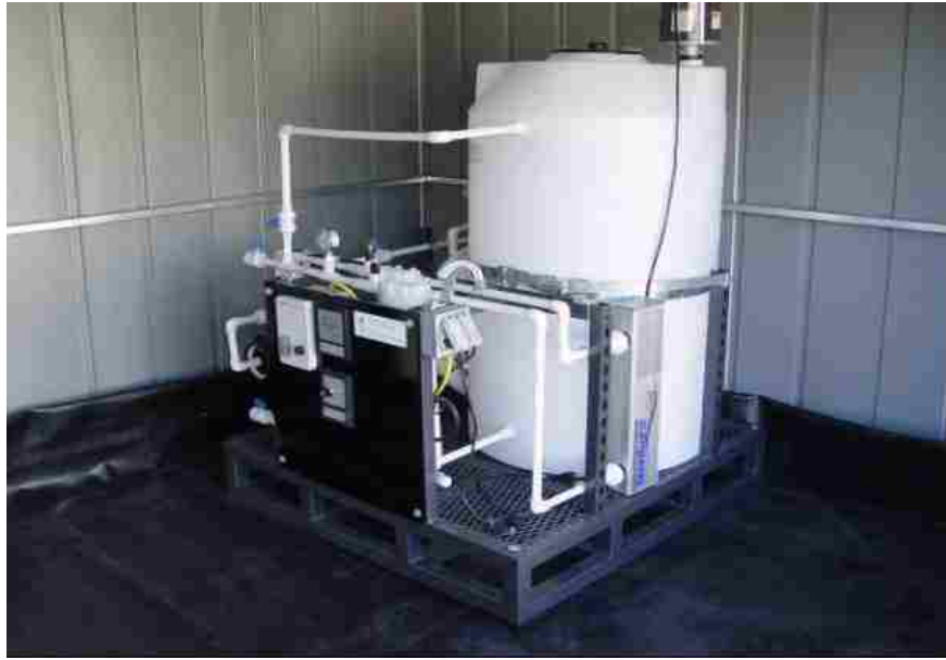
Figure 4.4: The water purification system used to provide optically pure water to the LTA for light transmission testing.
