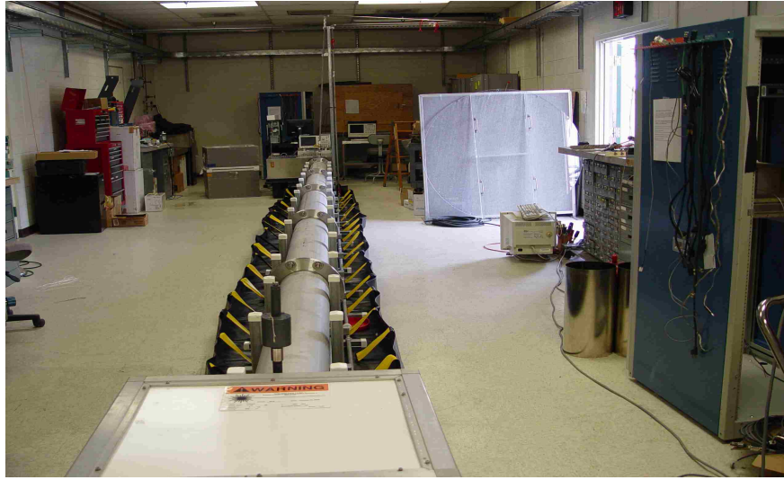
Figure 4.3: The LTA and associated optical benches. The laser beam is injected at the far end, traverses the arm, is reflected from a flat mirror in the mirror enclosure, and returns to the injection enclosure. The effective length is 20.08 meters
