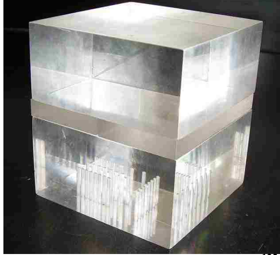
Figure 46: Photo of assembled PMMA phantom used in the ^{125}\text{I} calibration.
