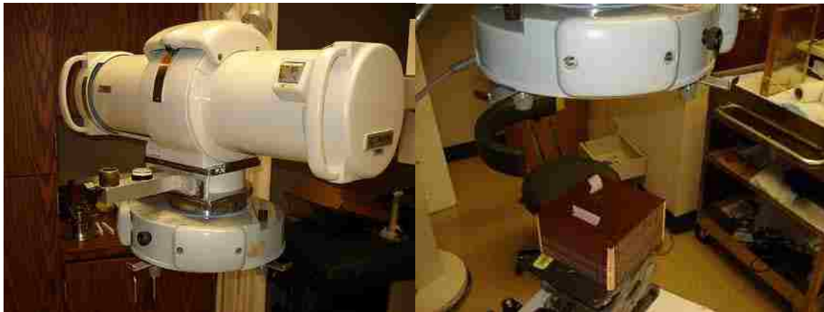
Figure 52: Left) Philips Orthovoltage RT-250 treatment head Right) phantom setup (Courtesy of MD Anderson Cancer Center).
