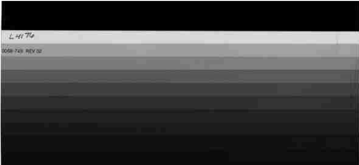
Figure 43: Kodak optical density photographic template used to transform Epson 1680 red-channel pixel values to optical density.
