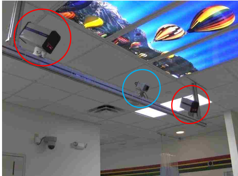
Figure 3.6: The infrared camera system mounted in the Novalis room. The red circles indicate the infrared cameras used for monitoring the external BrainLab bodymarkers. The blue circle identifies as an optical-light camera for visual monitoring.
