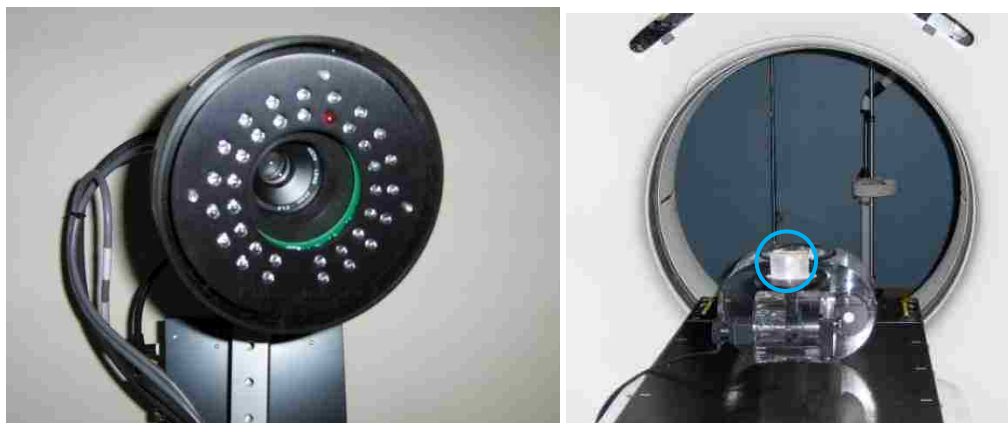
Figure 3.2: Varian RPM system 4DCT infrared camera mounted at base of CT couch (left) and the Quasar respiratory phantom affixed with the RPM marker box (blue circle) as seen from the camera's point of view (right)
