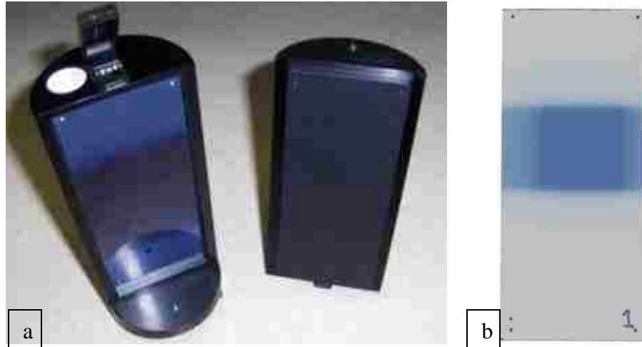
Figure 4.4: (a) Internal view of film canister with radiochromic EBT film in place and (b) sample film showing registration marks from Quasar film canister.
