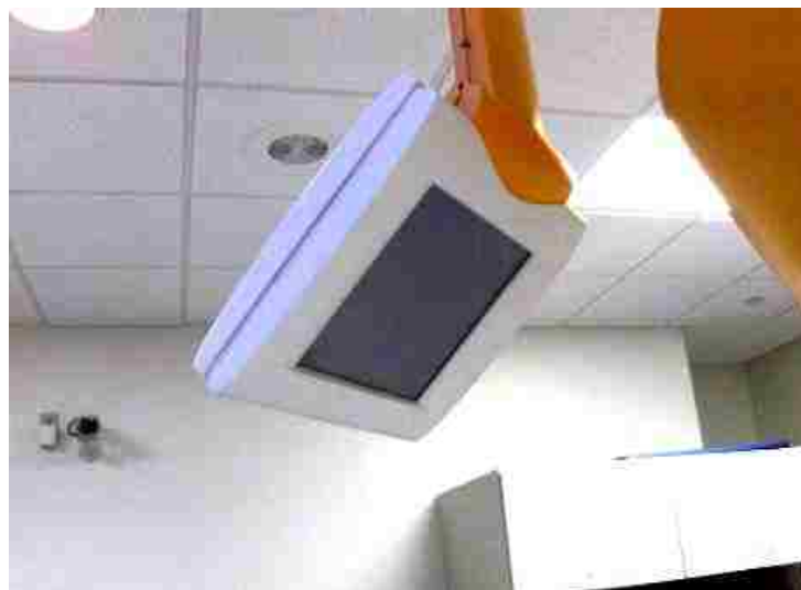
Figure 3.4: Picture of the ExacTrac amorphous silicon image detector mounted to the ceiling.
