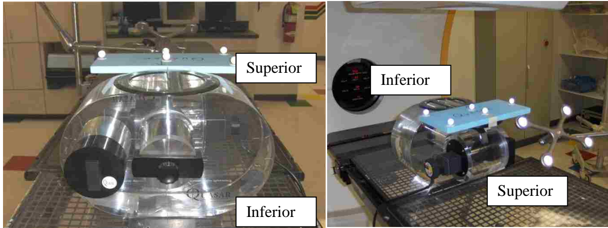
Figure 4.2: The Quasar phantom viewed from the gantry (left) and as viewed standing next to the foot of the couch (right). Labels denote the superior and inferior sides of the phantom.
