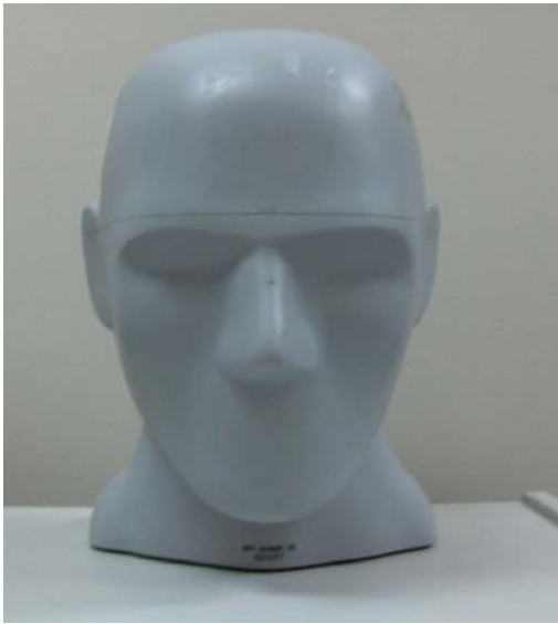
Figure 14. Photograph of CIRS model 605 radiosurgery head phantom.
