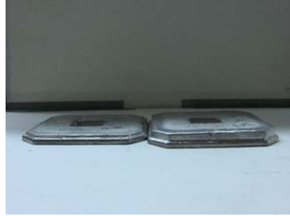
Figure 38. Photograph showing a 6 mm thick mask next to a 10 mm thick mask.
