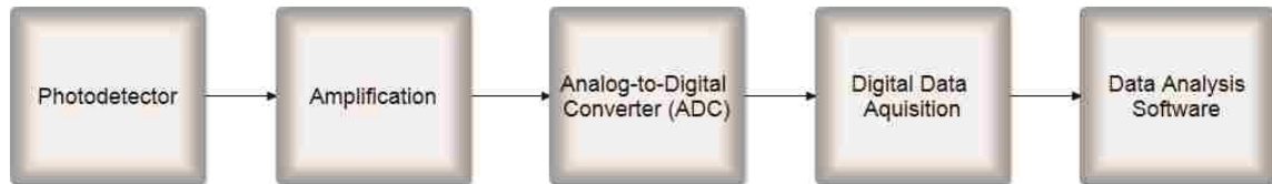
Figure 2: General flow of electronics and analysis of a modern flow cytometer
