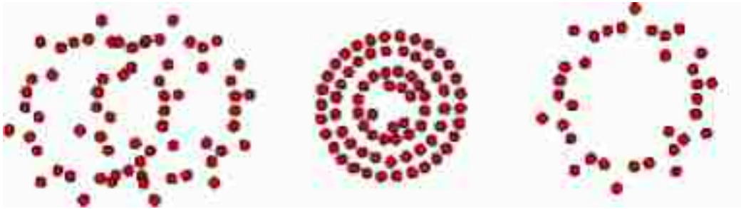
FIGURE 0.17. Hit topologies of electrons (left), muons (middle) and NC \pi^0 (right) events in the MiniBooNE detector.
