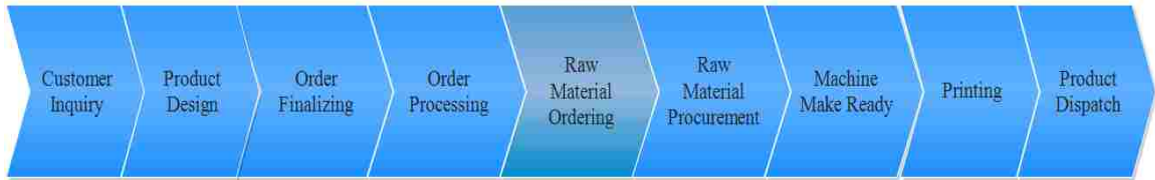
Fig 5: Traditional Printing Process – Process Flow (Konig, 2013)
